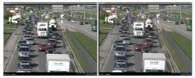
The image on the left was recorded at a bit rate of 2.5 Mb/s in MPEG4-SP, the one on the right at 1.5 Mb/s in H.264 Main Profile. Yet the quality of this image is higher. Details are more pronounced, edges are cleaner, and objects in the distance are clearer with more vivid colors.
