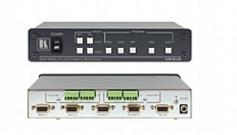
The VP-2x2 is a high-performance matrix switcher for computer graphics video signals, with resolutions up to and exceeding UXGA, and balanced stereo audio signals. It can route either or both inputs to either or both outputs simultaneously.
